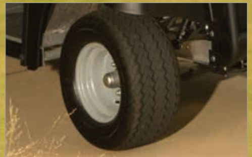
Turf-Friendly Tires: Bigger for more ground clearance, gentler on the turf.
