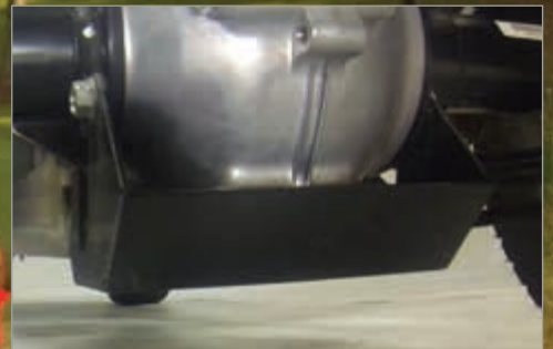
Differential Guard: Protects the differential from damage in rugged terrain.
